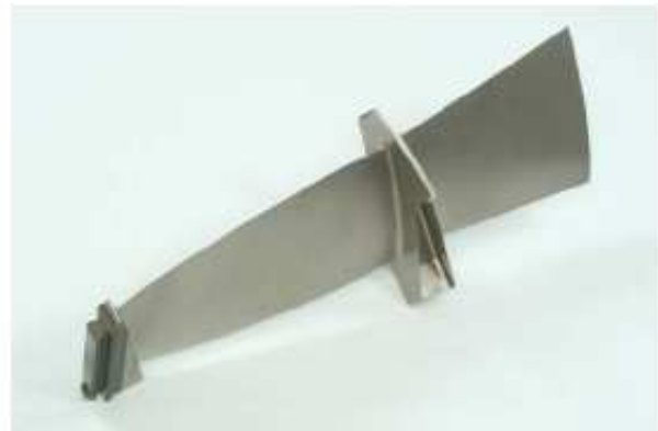
Fretting wear on titanium fanblade snubbers was increased from 100 hours to 30,000 hours by Detonation Gun™ application of a 0.25mm thick tungsten carbide-cobalt coating. Galling in the blade roots was eliminated electroplated copper-nickel-indium alloy. Courtesy Praxair Surface Technologies.
