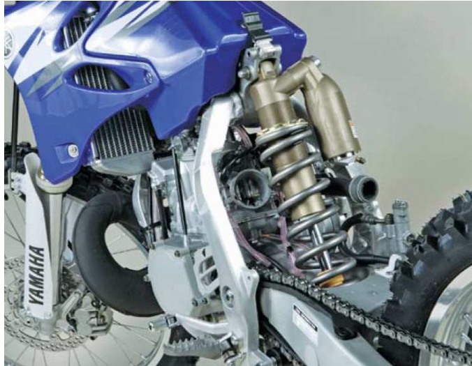
The TIMETAL LCB™ monoshock coil spring on the 2006 Yamaha YZ250 MX bike is 30% lighter than an equivalent steel spring
